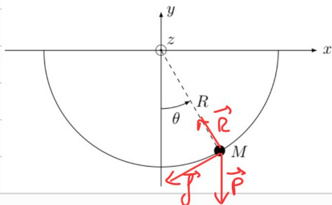
$$\begin{aligned}\vec{L}_0(n/R) &= \vec{on} \wedge m\vec{v}(n/R) \\ &= R\vec{u}_r \wedge mR\dot{\theta}\vec{u}_\theta = mR^2\dot{\theta}\vec{u}_3\end{aligned}$$
