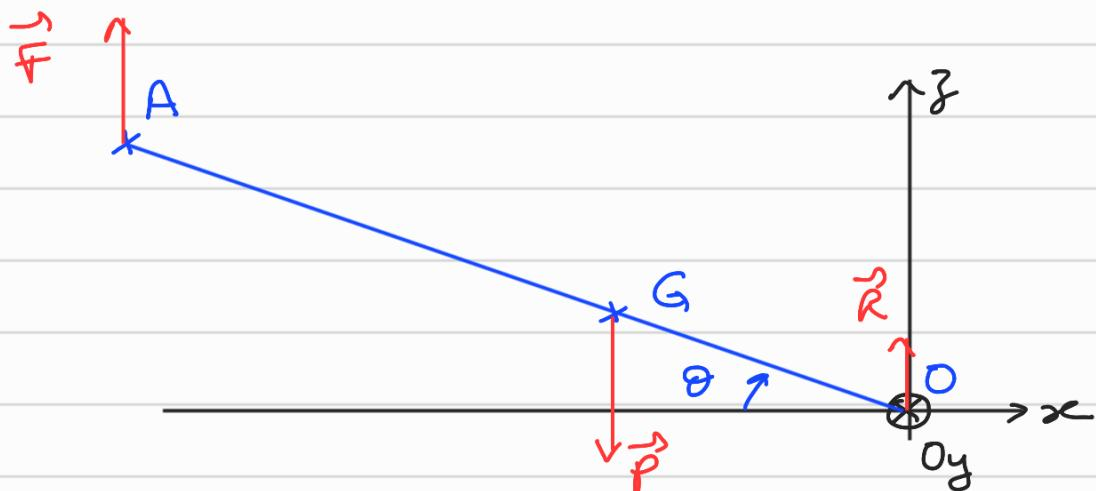
$$Q2. \frac{dL_{oy}(\text{mur})}{dt} = J\ddot{\theta}_{oy}(\vec{P}) + J\ddot{\theta}_{oy}(\vec{R}') + J\ddot{\theta}_{oy}(\vec{F})$$
