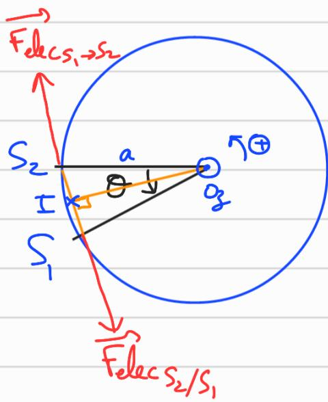
$$Q2. E_{p, \text{torsion}} = \frac{1}{2} C (\theta - \theta_b)^2 = \frac{1}{2} C \theta^2$$
