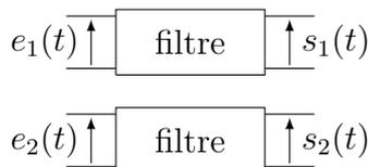
$$e(t) = \alpha e_1(t) + \beta e_2(t) \quad \xrightarrow{\text{filtre}} \quad s(t) = \alpha s_1(t) + \beta s_2(t)$$
